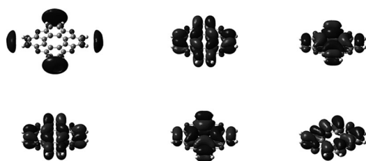
Figure 7. LUMO (top) and HOMO (bottom) density plots for tetraoxa[8]circulene with charge state -2 (left), 0 (middle) and +2 (right).
