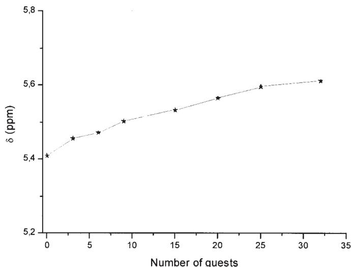
**Figure 5.**  $^1\text{H}$  NMR titration of dendrimer **5** with sulfonic acid guest **1**. The chemical shift of the urea protons in the host changes gradually upon the addition of the guest.
